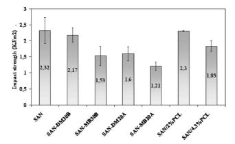
Fig. 5 Impact properties (Charpy) of SAN, SAN/clay nanocomposites (3 wt% clay) and SAN/PCL binary mixtures.
