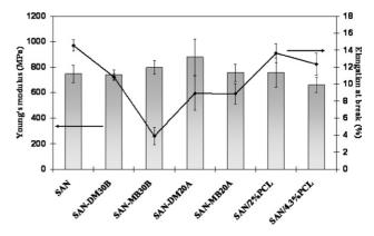
Fig. 4 Tensile properties of SAN, SAN/clay nanocomposites (3 wt% clay) and SAN/PCL binary mixtures.
