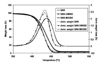
**Fig. 7** Thermogravimetric analysis curves of SAN and SAN/clay nanocomposites (3 wt% clay) under helium, at 20 °C min<sup>-1</sup>.
