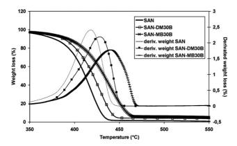
**Fig. 6** Thermogravimetric analysis curves of SAN and SAN/clay nanocomposites (3 wt% clay) under air, at 20 °C min<sup>-1</sup>.
