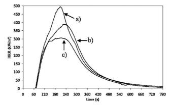
**Fig. 8** Cone calorimetry curves (heat flux: 35 kW m<sup>-2</sup>) corresponding to a) SAN, b) SAN-DM30B and c) SAN-MB30B.
