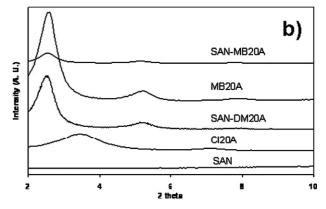
Fig. 3 XRD patterns of SAN, Cloisite® 20A, Cloisite® 30B, and SAN/clay nanocomposites containing 3 wt% of clay (inorganic fraction).
