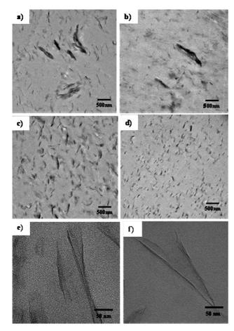
**Fig. 2** TEM images of SAN/clay nanocomposites containing 3 wt% of clay (inorganic fraction): a) SAN-DM20A, b) SAN-DM30B, c) SAN-MB20A, d) SAN-MB30B, e) SAN-MB20A (higher magnification), and f) SAN-MB30B (higher magnification).
